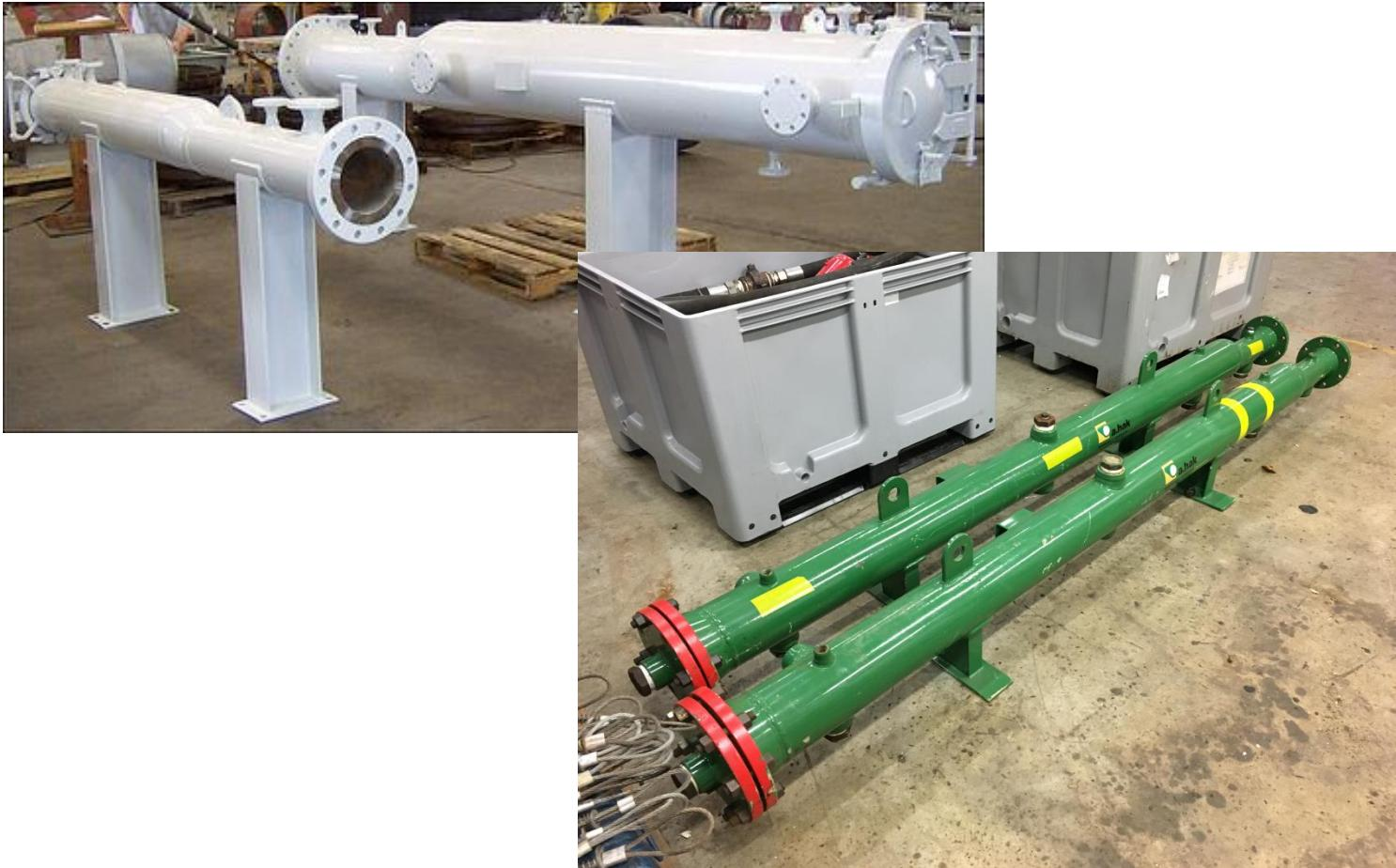
Pig launcher and receiver
