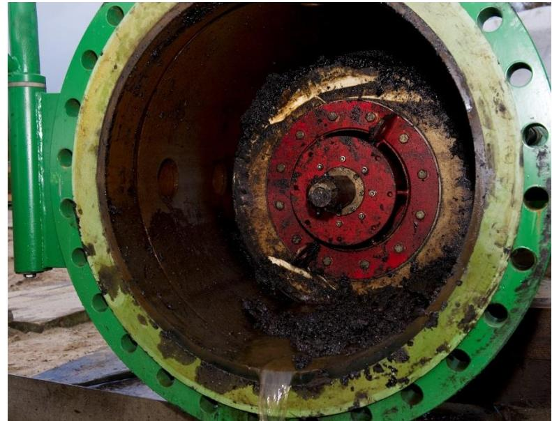
Debris, wax, scale, rust, sand, etc...
