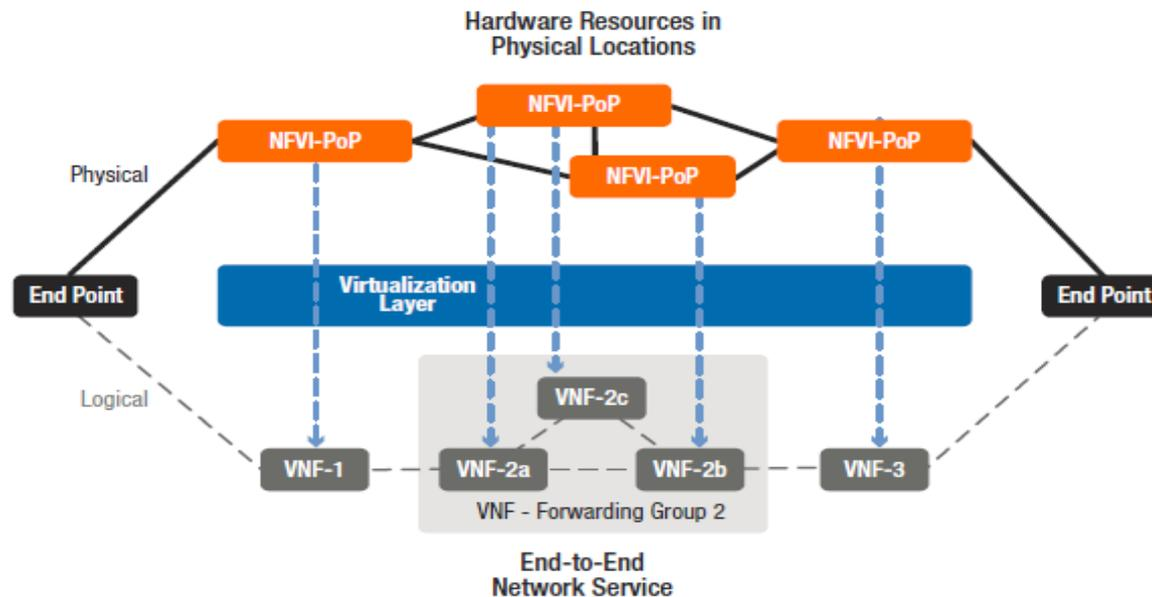
Figure 4. End-to-end network service. (original source: ETSI [www.etsi.org/deliver/etsi\\_gs/NFV/001\\_099/002/01.01.01\\_60/gs\\_NFV002v010101p.pdf](http://www.etsi.org/deliver/etsi_gs/NFV/001_099/002/01.01.01_60/gs_NFV002v010101p.pdf))
