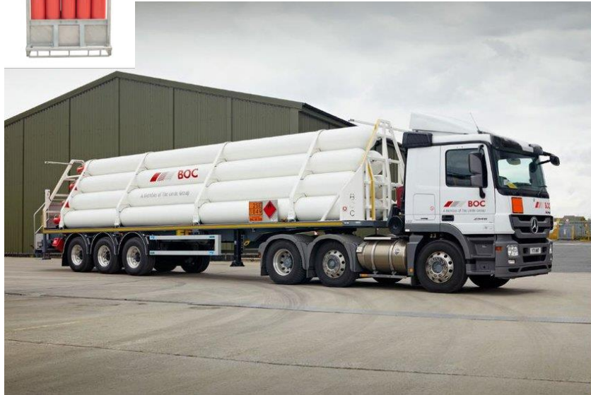
Conventional steel tubes (tube trailer) 200 bar – 300 kg hydrogen
