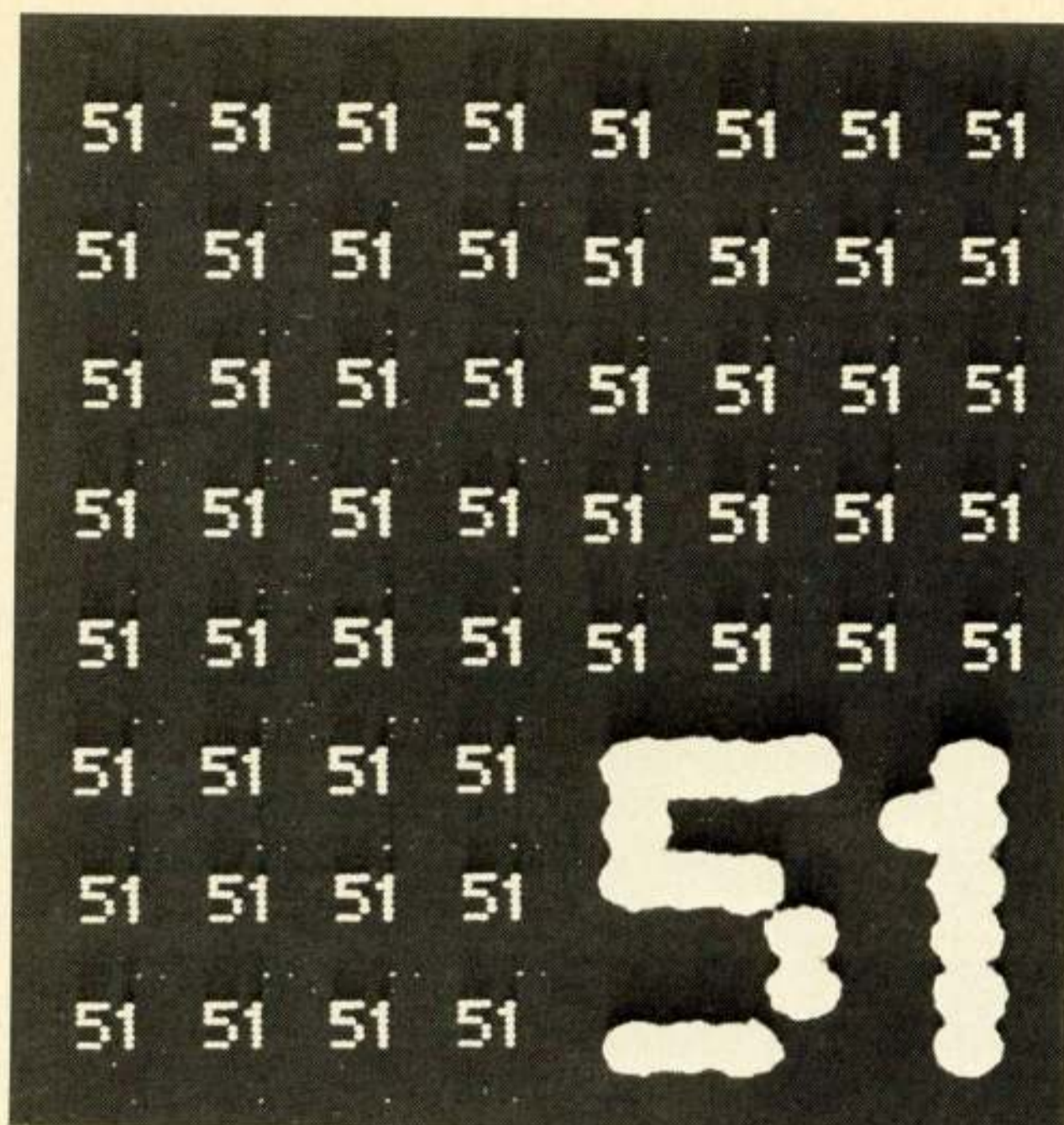
Fig. 1. Display of symbols by a random-access method. Inserted in the lower right-hand corner the display in detail is shown of number 51.
