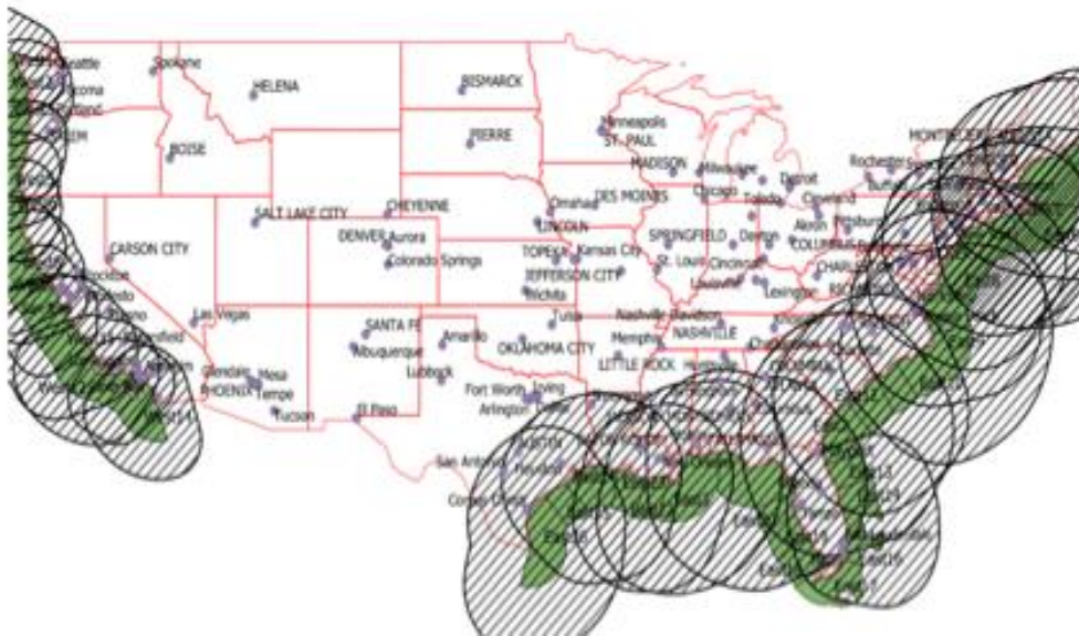
Figure 5: Dynamic Protection Areas in CBRS and their neighbourhoods that require ESC-coverage for category B (outdoor) operation.
