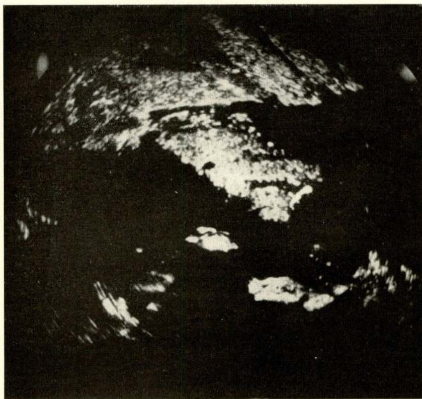
Fig. 3. Radar picture of Bergen (Norway) 3.20 cm radar, d/r \sim 1/50 , S \sim 3000 m.
