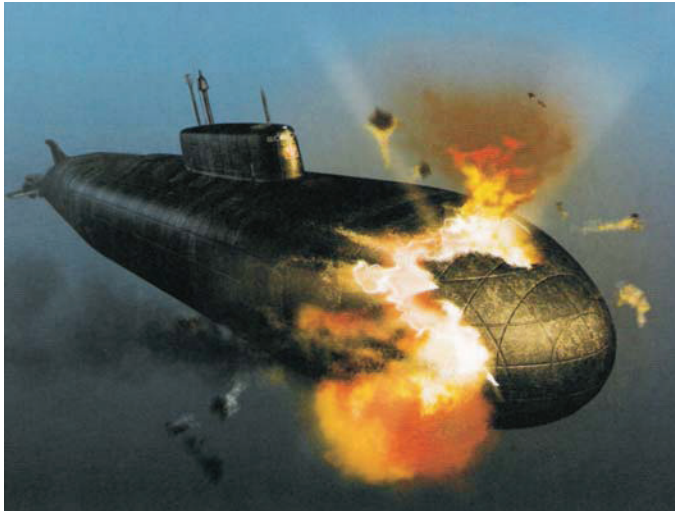
Figure 2: The explosion occurred in the foremost compartment, where the torpedoes were stored. The depth the sub was at prevented the shockwave from forcing its way out of the sub; instead, most of the force of the blast traveled through the vessel's interior, causing devastation.
