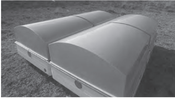
Fig. 1. Four THEA tiles in a compact setting, covered with the protecting radome
