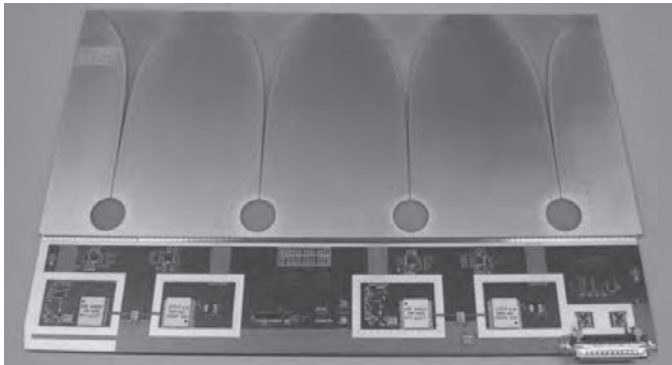
Fig. 2. A picture of a column board, with 4 antennas, amplifying and beamforming network
