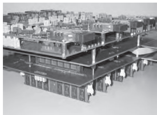
Fig. 4. Photograph of the High Speed Link Receiver, the Digital Beamformer and the Selection board
