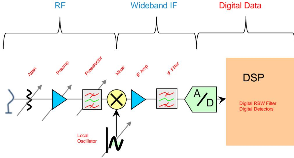
**Wideband IF** into ADC and digital signal processing via dedicated **FPGA** provide for a entire new level of feature / functionality including:
