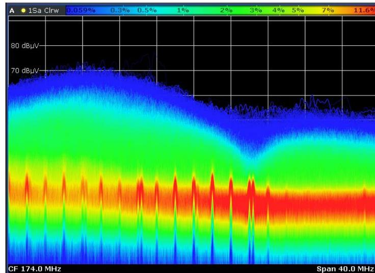
2nd pulsed disturbance signal hidden by the broadband noise, not detectable by conventional spectrum analysis
