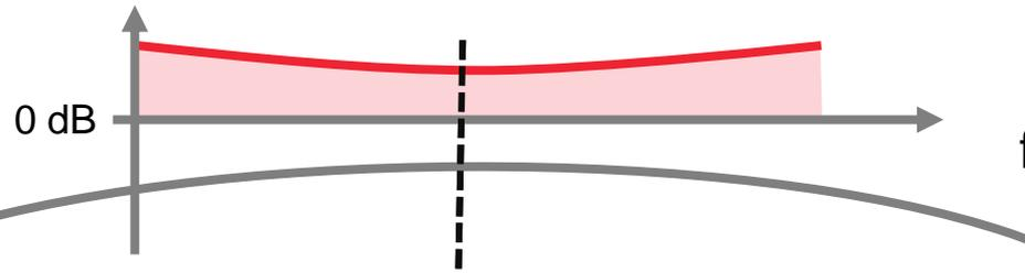
Compensation of previous level reduction caused by last stage IF filter.
