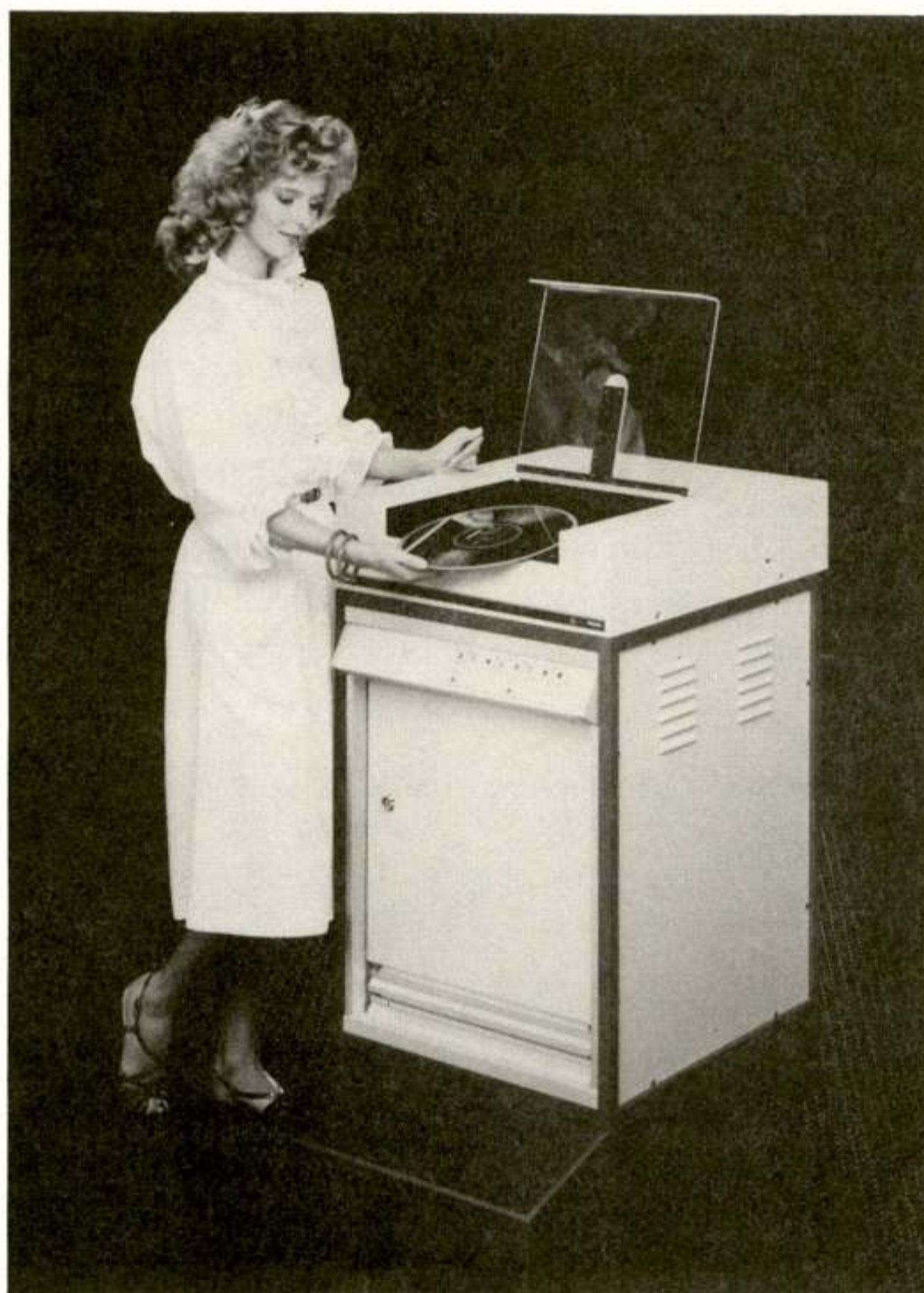
Figure 1: The diode laser based digital optical recorder is able to access 1,000 M bytes
