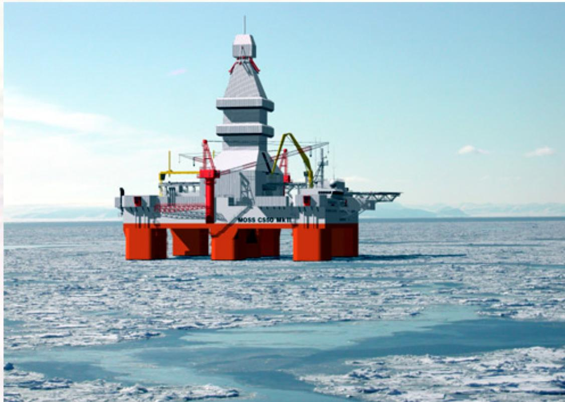
Artist impression of a dynamically positioned semi-submersible rig
