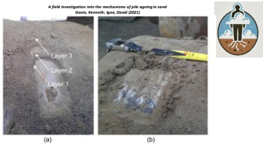
Fig. 15. Photographs of cemented sand crust adhered to pile S6 following extraction: (a) cemented sand crust on pile with distinct layers; (b) difficulty removing layer 1
