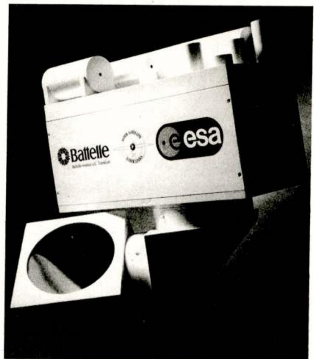
Fig. 8: Wooden mockup of the transceiver package. On the top level, one can see from foreground to background: LO laser, modulator head, transmitter laser. The device attached underneath the package is the Coarse Pointing Assembly of the PAT.
