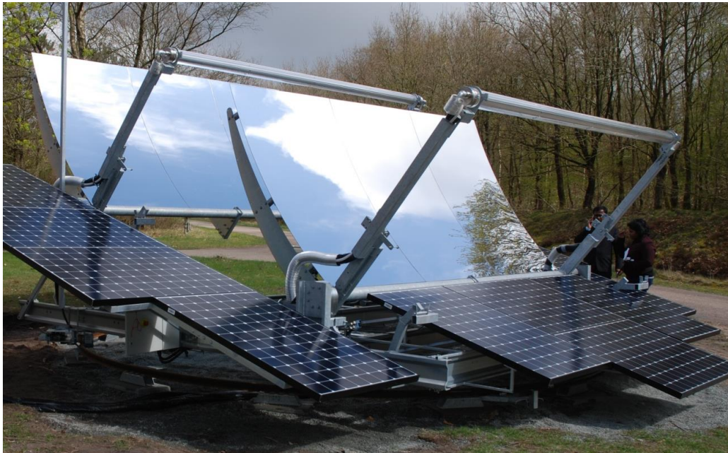
SunOyster with additional 12 PV modules
