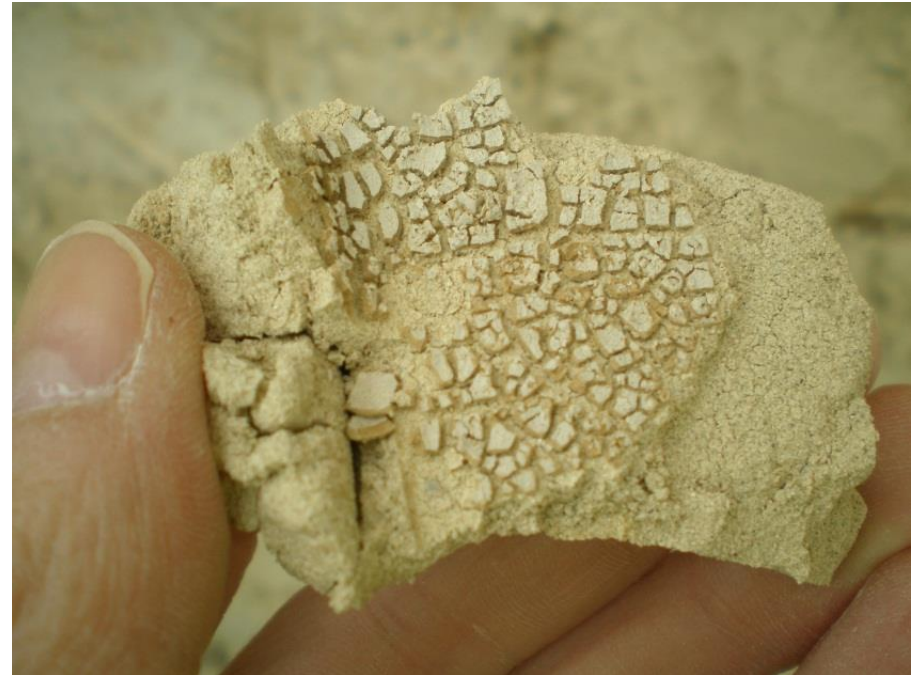
Filtercake, as peeled from a D-wall
