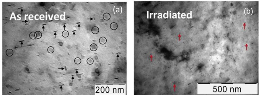
High density fine precipitates throughout the microstructure of irradiated specimens
