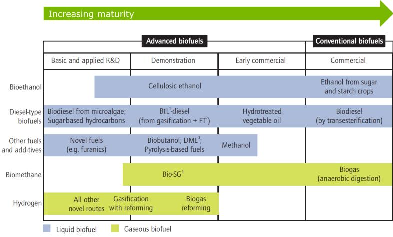
1. Biomass-to-liquids; 2. Fischer-Tropsch; 3. Dimethylether; 4. Bio-synthetic gas.
