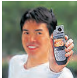
Fig. 1 Example of a Japanese I-mode terminal, which has a built-in videocamera. I-mode works over the GSM-like PDS system. The I-mode terminals are a prelude to the terminals (and services) that will be possible with UMTS.
