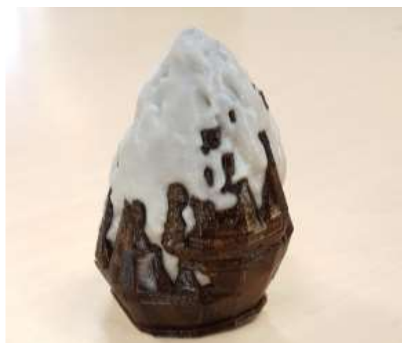
figure 2 Second printed prototype (ABS with support materail).
