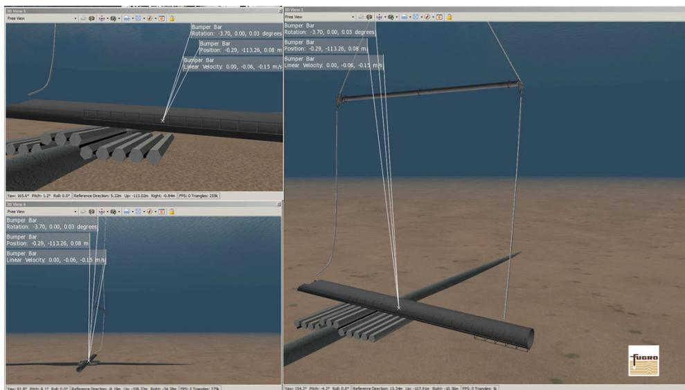
Simulation raising a failed bumper bar from the seabed to **mitigate risk** of a potentially hazardous situation.
