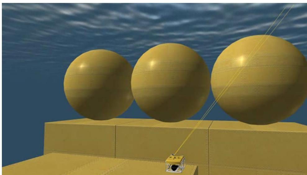
Simulation to review the blind spots on the sonar display as a result of the introduction of a protective frame on the ROV.
