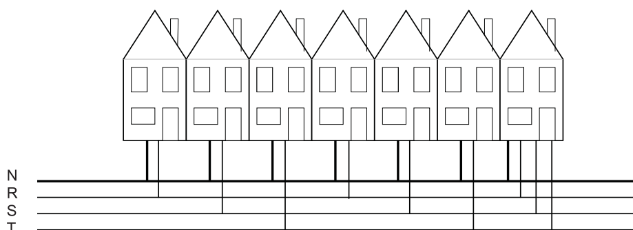
Figure 9: Common power supply lay out on street level.
