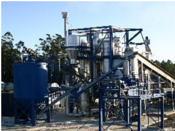
FLUIDISED BED GASIFIERS Clean technology suitable for 'difficult' fuels.
