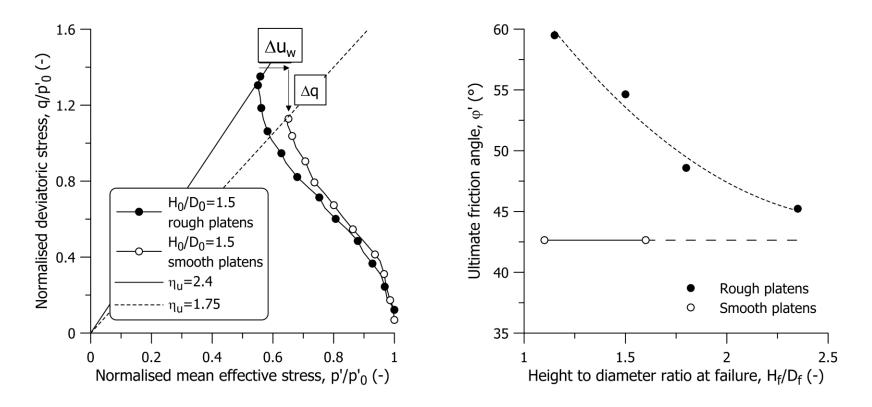
• Bias in the ultimate friction angle  $\phi$ '= 55° to  $\phi$ '= 42°
