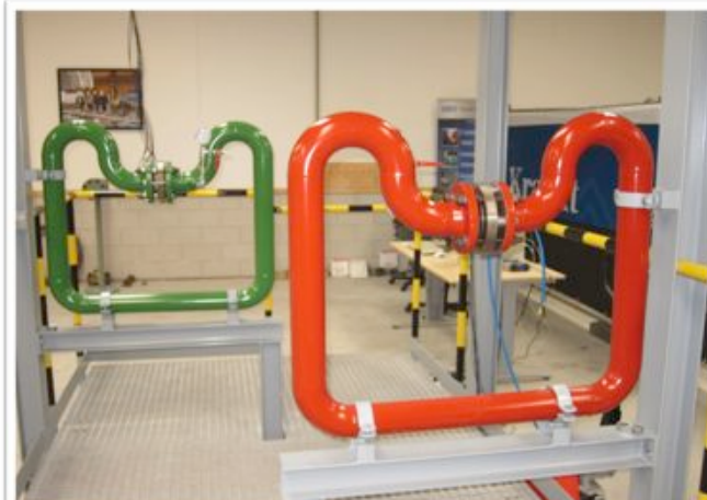
'Piping training skid' – flens 'misalignment' Groene leiding: flens = 2° 'angular misalignment' Rode leiding: flens = 20 [mm] 'cold pull'
