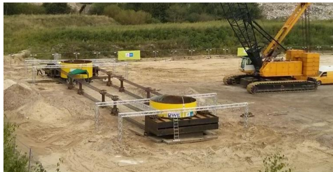
lateral load test
