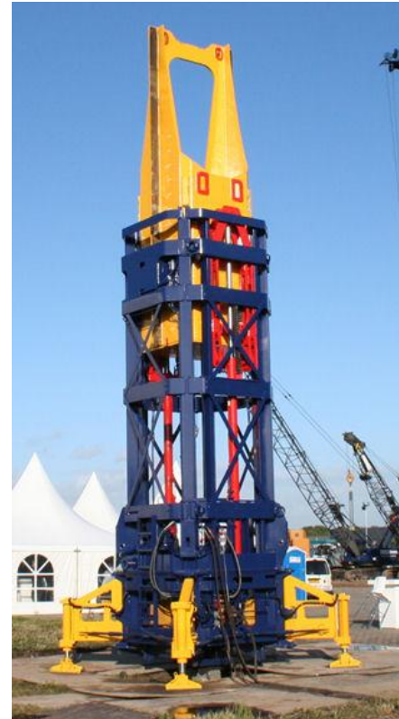
rapid load test (RLT)
