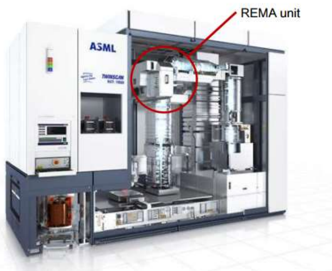
REMA unit inside a lithography machine
