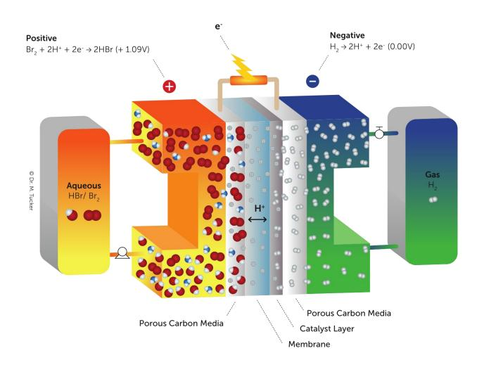
discharge: fuel cell  $H_2 + Br_2 \longrightarrow 2HBr + Electrical energy$ charge: electrolyser
