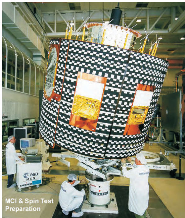
Figure 5: MSG Satellite with Antenna Farm on top (Qualification Model, courtesy Alcatel)
