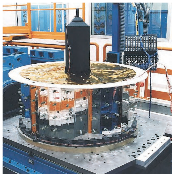
Figure 8: L-Band EDA with S/L TPA and TTC antenna on top, before environmental testing (courtesy Alenia)
