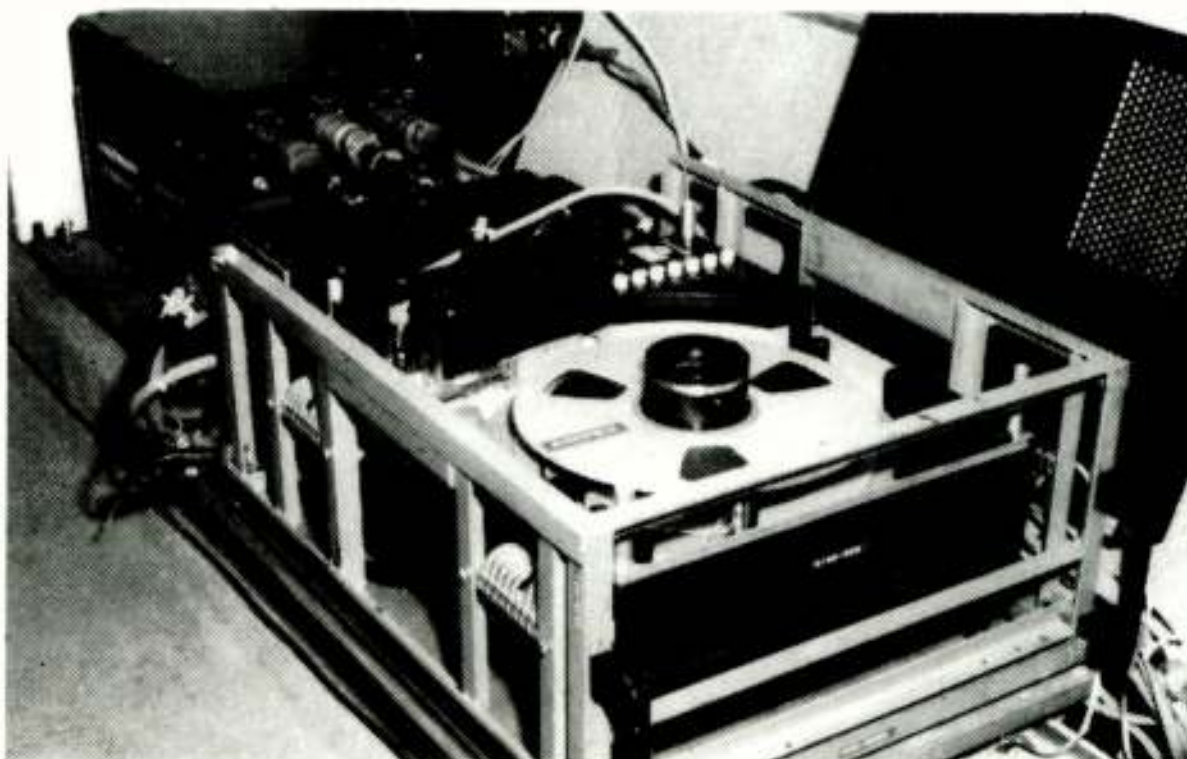
Figure 3. High Bit Rate interface and High Density Digital Tape recorder in the aircraft.
