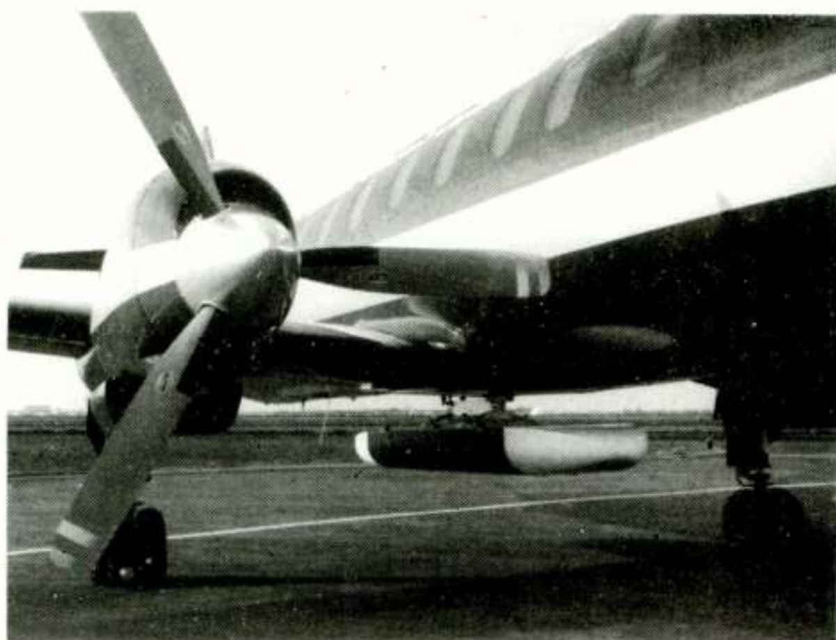
Figure 5. The antenna of the SLAR under the aircraft
