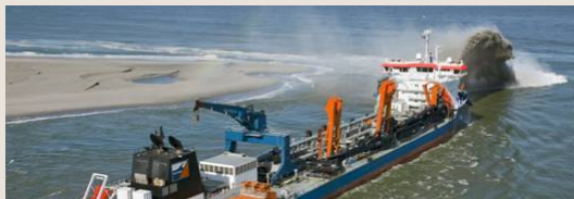
Custom-built tralling suction hopper dredger: VOX MAXIMA
