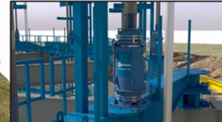
synchronized lifting by means of strandjack system
