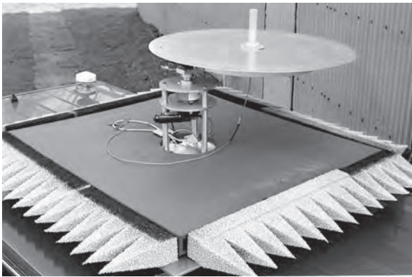
Fig. 2. Rotating antenna on top of the measurement vehicle.
