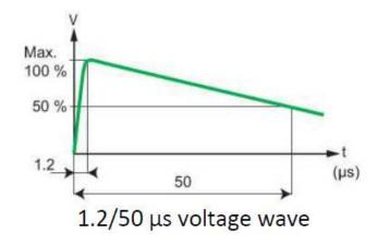
This type of voltage wave is used to verify equipments ability to withstand voltages of an atmospheric origin.
