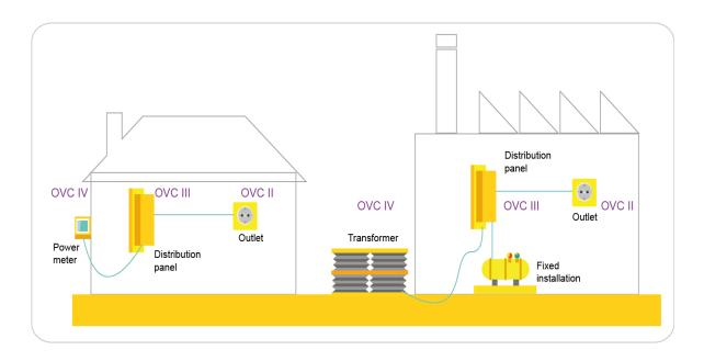
OVC III Equipment is downward compatible with OVC II, I application and environment.
