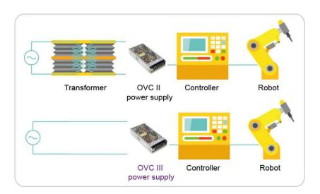
Some robot controller products to meet the IEC60204-1 standard need an additional AC transformer in series between the power grid and power supply
