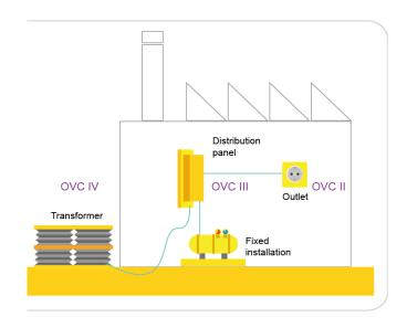
OVC III is equipment in fixed installations and for cases where the reliability and the availability of the equipment is subject to special requirements.
