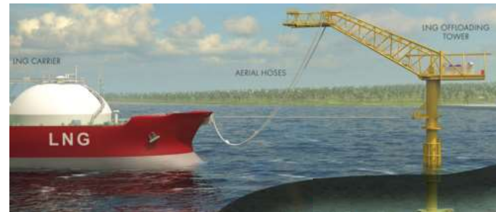
Cryogenic loading tower
