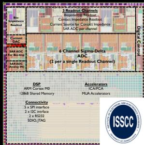
Multi-parameter Interface & Embedded Signal Processing For connected health
