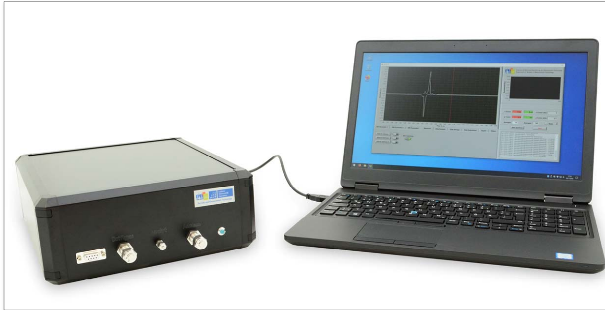
Closed gas loop GC-IMS (not size optimized)
