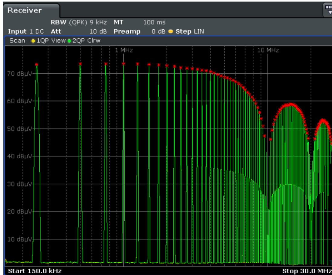
Fig. 16: Measured signal spectra, quasi-peak detector, 150 MHz to 30 MHz.
