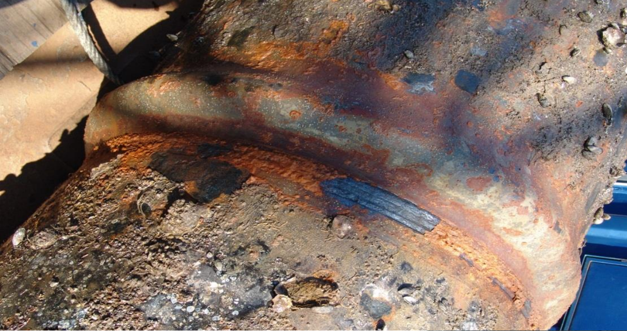
Local buckling sand filled tube (outwards)
