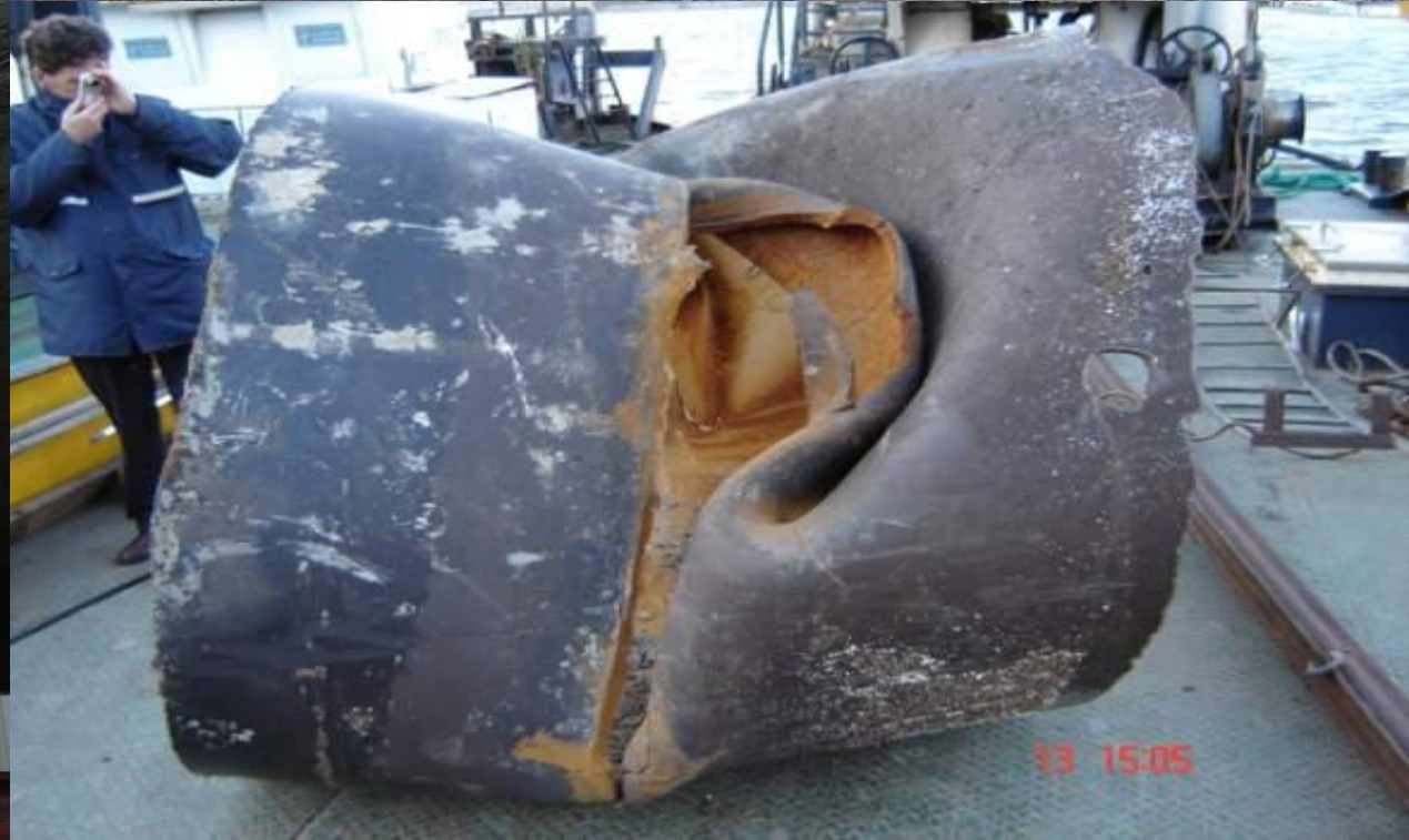
Local buckling empty tube (inwards)
