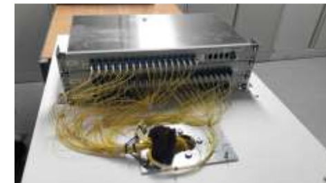
+ (C+L band) AWGR, 144 ports, \Delta\nu=50\text{GHz} , BW_{-3\text{dB}}=35 (/24)GHz
