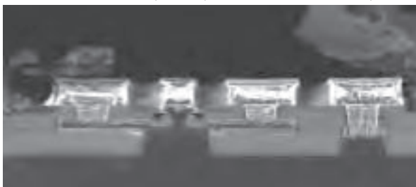
Figure 7. Modern self-aligned SiGe heterojunction bipolar transistor (HBT) in 0.18 um technology. The contacts are from left to right Base-Emitter-Base-Collector, and typical contact size is 1 um. Two base contacts are used to reduce the series resistance in the base contact. (courtesy Philips Research Leuven).
