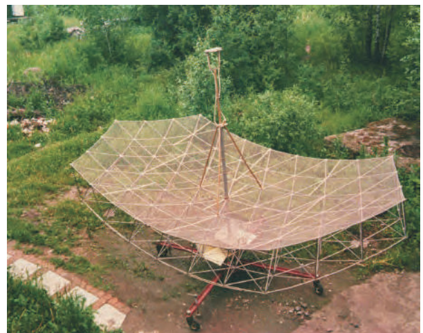
Figure 2: TRAVERS antenna, used for L-S band SAR on Priroda (MIR), courtesy OKB-MEI
