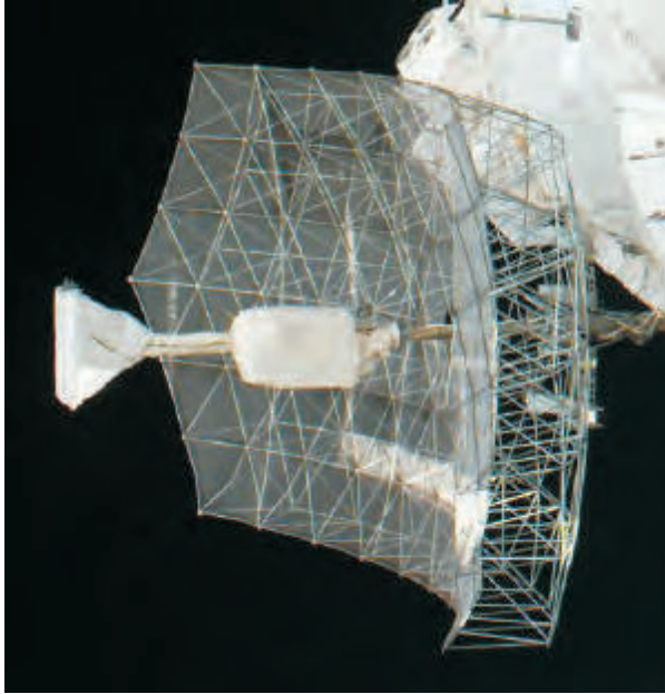
Figure 4: Antenna of the L – S band SAR on the Priroda platform on MIR (+).
