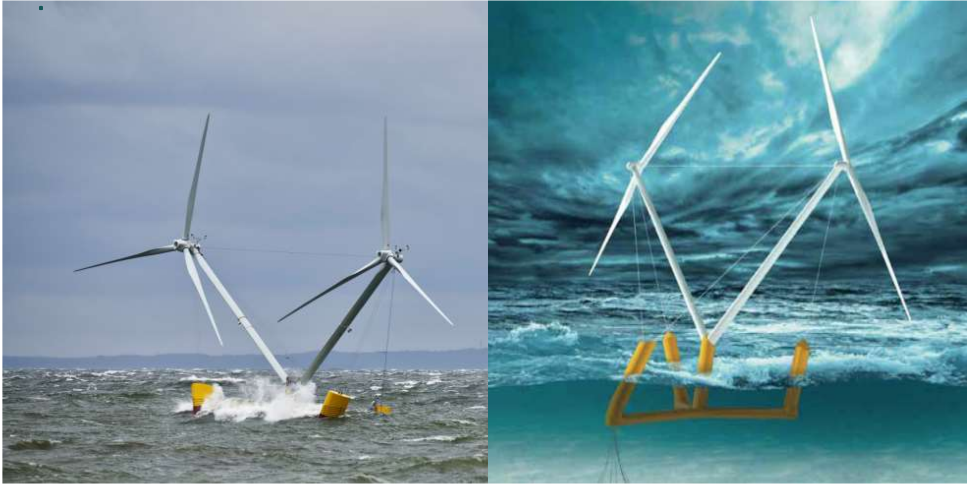
Nezzy 2 floating offshore platform (1:10) in the Bay of Greifswald in the Baltic Sea
