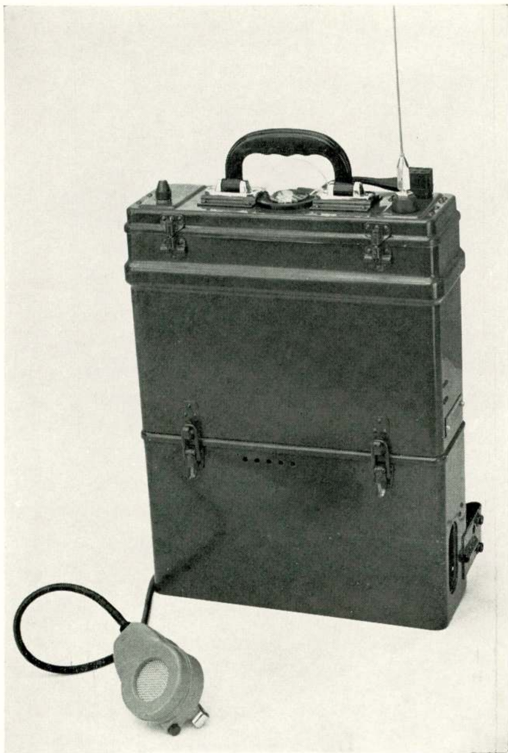
Fig. 1 Packset SDR 314, with immersion proof microphone
