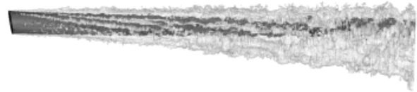
Fig. 5: Visualization of the interfaces between gas and spray (VOF=0.01) and spray and liquid (VOF=0.99); Eccentric located orifice leading to a wrinkling up and rotation of the core
