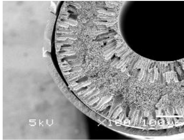
Delamination because of insufficient adhesion between coating and support.
