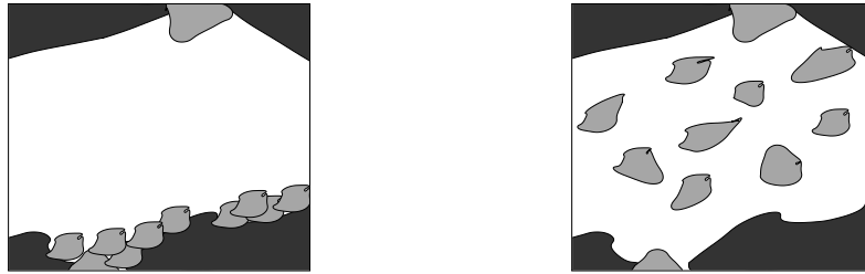
Figure 6.4.1: Expansion of the fine fraction. Without flow (left) the fine grains are present as a layer on the bottom of the pores in the coarse matrix. When the fines are mobilised, but not yet transported due to larger fines clogging the pore constrictions, the fine fraction occupies a greater area in the FOV (right).
