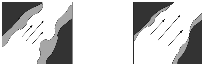
Figure 6.4.2: No fluid flow within the fine fraction (light coloured) leads to erosion at the interface between the fluid (white) and the fine fraction.
