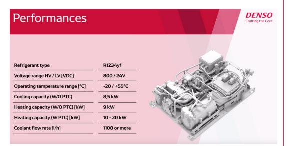
Stand alone device to heat and cool the battery by using heat pump system, typically used Off Road and Special Applications
