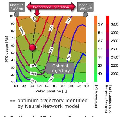
→ Optimal efficiency found at intermediate valve position
